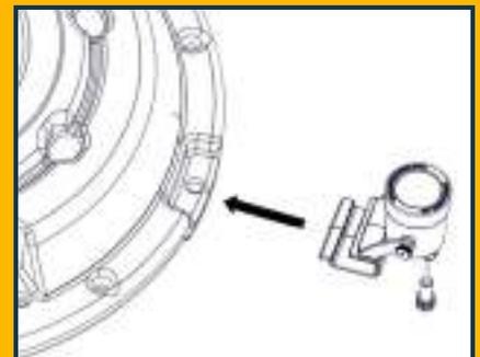
Snap-on clips included with RGB, Composite LED, and Stainless Steel LED systems.
